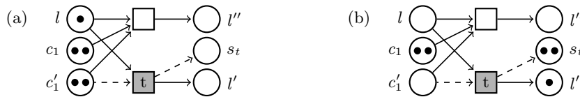
Fig. 3. A Petri net with transfer modelling a test for zero in a counter machine. Dashed lines represent transfer arcs of t that move all tokens in c'_1 to the trash place s_t .
