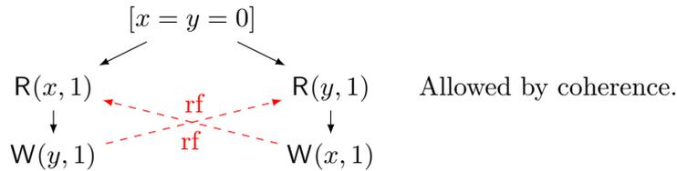
Note that there is a cycle in  $po \cup rf$  in this example, but this cycle is not forbidden by the coherence axioms because it involves two different locations.
