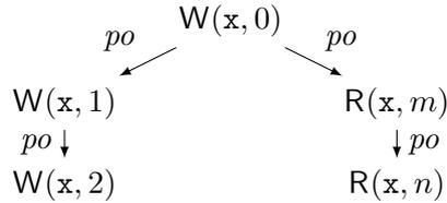
for every possible  $m, n \in \text{Val}$ . Obviously not every such execution is a valid run of the program. It is the memory model that will constrain the set of ‘valid’ executions by providing a number of constraints (axioms).
