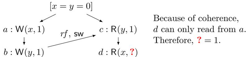
**Store buffering example** It is worth pointing out that release-acquire is weaker than sequential consistency (i.e., the usual interleaving semantics), as illustrated by the *store buffering* (SB) example below. The program is the following:
