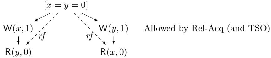
This relaxed behaviour, however, cannot occur under any interleaving of the two threads. The reason is that in any interleaving, one of the threads has to start before the other, and therefore its write will happen before the corresponding read of the other thread.
