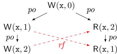
(Note that although  $rf$  is a function from reads to writes, when depicting it as a relation, we point the arrow from the write to the read, because the write is logically before the read in time.)
