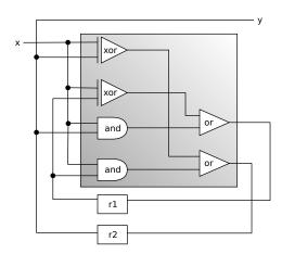
The circuit uses registers  $r_1$  and  $r_2$ , which are initially  $r_1 = 0$  and  $r_2 = 1$ .
